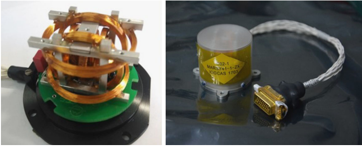
Fig. 2 The structure (left) and the packaged appearance (right) of RoMAG sensor
