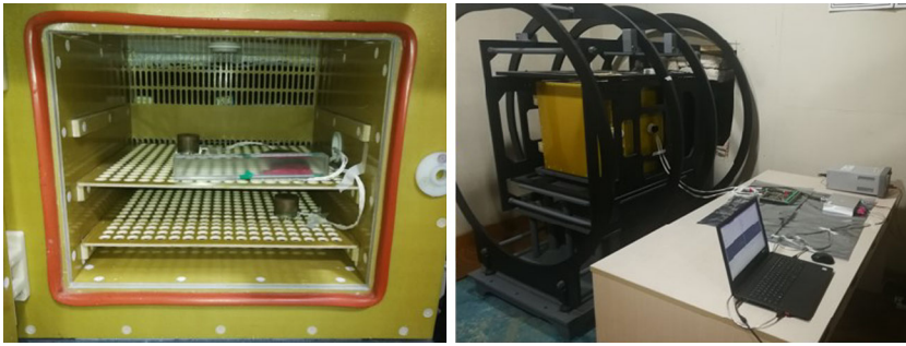
Fig. 7 The thermal box with a coil system
